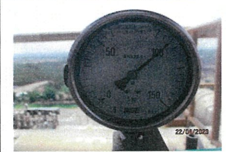
Hydrostatic Pressure Test HP LOOP
