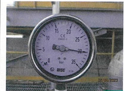
Hydrostatic Pressure Test IP LOOP
