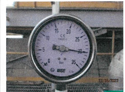
Hydrostatic Pressure Test IP LOOP
