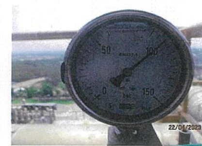
Hydrostatic Pressure Test HP LOOP
